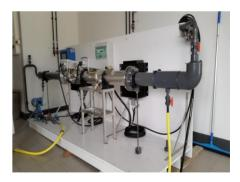
HOD system successfully inactivate OsHV-1 and Vibrio
